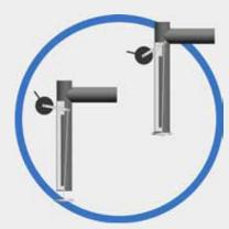
The automatic shut-off valve closes the outlet pipe when the maximum oil storage capacity is reached.
