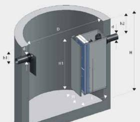
ecoLine-b offers a full range of below ground oil water separators from 50gpm (3l/s) to 320gpm (20l/s). Larger models are available upon request. Grit chamber shall be sized depending on the particular application.
