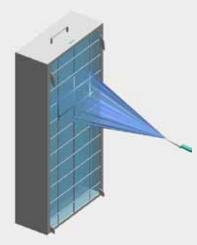
The coalescing media cartridge has to be cleaned periodically. Since the maintenance intervals strongly depend on the particular application, check the condition of the filter element weekly during the first 60 days of operation. The filter media can be cleaned/rinsed with a garden hose. Recycle the wash-water to the separator. Do not expose the media to sunlight or UV-radiation for extended periods of time. Remove sludge and oil from the system periodically.
