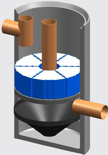
**Freytech presents ecoStorm plus, an affordable stormwater filtration system designed to remove sediments, heavy metals and nutrients.**
